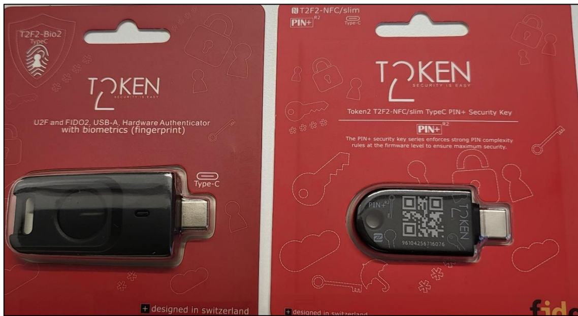
Fig 1: Hardware token in the form of USB sticks: fingerprint token (left) and password token (right).
